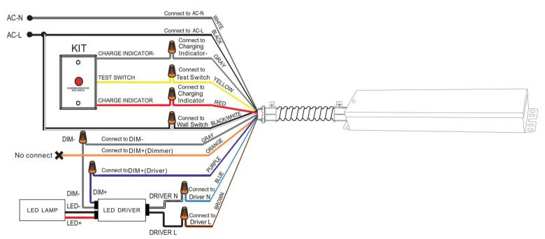
Note: Utilize wire nuts to secure any unused wires.
