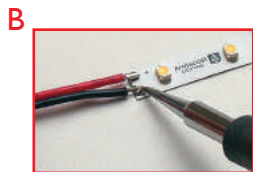
B: Terminated ends can be soldered to with standard 50/50 rosin core lead solder.
