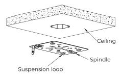
iii. Connect the clip on the fixture to the spindle of the mounting plate to make sure the fixture will not slip and fall. Connect the line voltage to the wires coming out from the fixture following the wiring diagram. Push the pressing plate into the suspension loop on the mounting plate.
