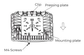
ii. Fix the mounting plate to the ceiling with the screws.
