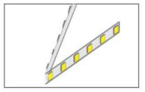
Do not fold or crease LED Strip light, , and this way will break the LED and bonding pad
