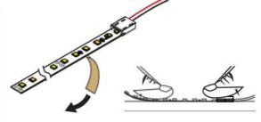
Remove the 3M tape from the connection and Ensure ambient temp is minimum 50 ° F (10 ° C) or tape will not adhere properly. Attach the strip to the installation position, and Adhere to a smooth, dry surface, working one end to the other.
