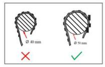
Do not bend LED Strip light to a diameter less than 40mm(1.5 inches)
