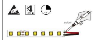
Connecting two welded parts with a maximum temperature of 250 ° C and no more than 5 seconds, and you must wear an electrostatic bracelet,
