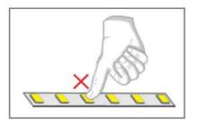
Do not put press heavily or put excessive pressure on surface of LED
