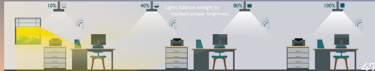
DAYLIGHT HARVESTING SENSORS AND DIMMING POWER PACKS BALANCE EFFECTIVE LIGHT AND SAVE ENERGY
