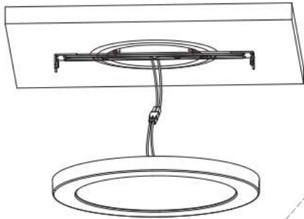
A. J-Box installation is applied to 6W/12W/18W/24W mini panel for North American market
