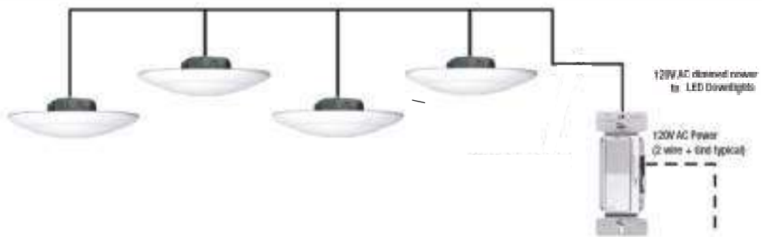
Figure 2 Junction Box Installation
