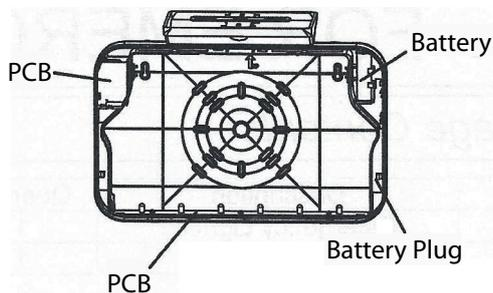
6. Snap fixture onto mounting plate and ensure no wires are pinched. Make sure until is fully attached.
