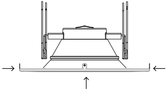
3. Flatten the four clamps to secure the trim to the fixture.
