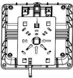
2. Connect the wires threaded from conduit and Canopy, Black wire for Line, White for Neutral, Green/Yellow Green for Ground.
