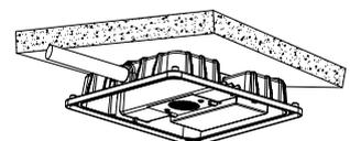
4. Disconnect the wires came from 3/4" hole and connect the wires came from 1/2" conduit with canopy . (White for Neutral, Black for Line, Green/Yellow Green for Ground)
