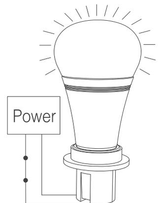
**3** As soon as the light has power, and while it is flashing, quickly press any "Zone ON" button 3 times within 3 seconds. This assigns that device to the chosen Zone. Multiple devices can be controlled in the same zone
