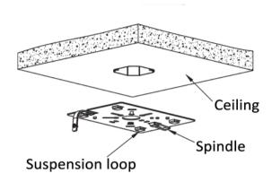
iii. Connect the clip on the fixture to the spindle of the mounting plate to make sure the fixture will not slip and fall. Connect the line voltage to the wires coming out from the fixture following the wiring diagram. Push the pressing plate into the suspension loop on the mounting plate.
